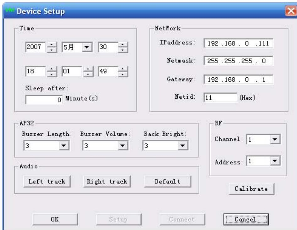
For the TL-3000 wireless touch panel, the main settings of the device are as follows, including IP address, system clock, sleep time, length of buzzer, volume of buzzer, brightness of back light, volume of audio output (left and right channels), wireless frequency, local wireless ID address, etc.
