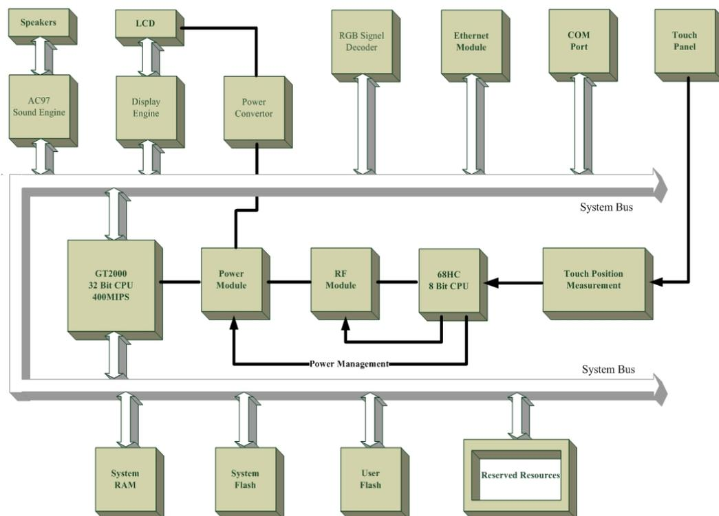
As shown in the diagram, the TL-3000 wireless touch panel comprises a series of high performance chips and IC's in clear and reasonable structure. The core of the system is a robust embedded 32-bit CPU and an auxiliary 8-bit CPU. The system expands its multifunctional interfaces through high-speed bus and offers the capacity of processing all types of information at high speed as image processing and network information is directly connected to the CPU bus
